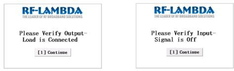
Please follow the instructions on the front panel LCD screen after switching on the power. Press "1" on keypad to continue.
