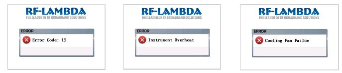
The front panel LCD screen will display the error code or error message when instrument self protection is triggered. Front panel alarm indicator will light up.
