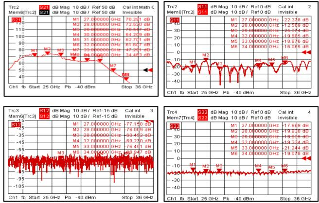
Note: Input/output return loss measurements include attenuators to protect equipment
